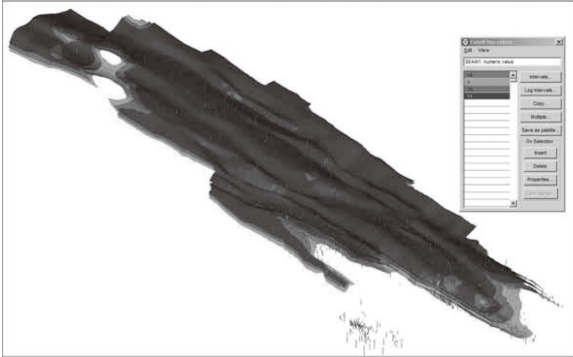
Figure 7.11 3D Isometric View (NW) of No. 9 Area Coal Seams, Faults and Drillholes
