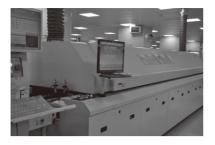
• Solder parts and components onto PCB by soldering machines
