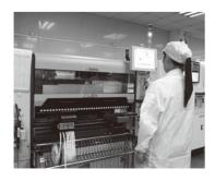
• Fix surface mount device (SMD) components onto PCB by SMT machines
