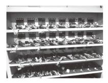
Load and test the switching power supply unit for consumer products and smart charger and controller for industrial use for a few hours
