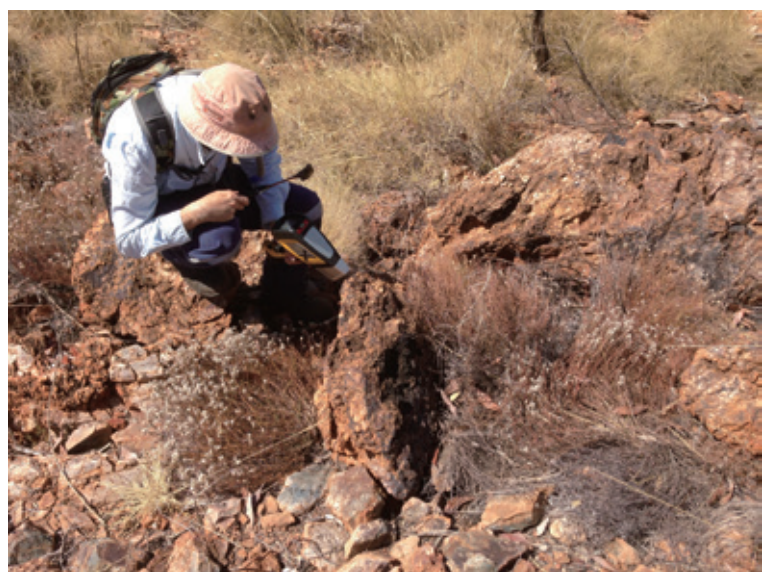
Figure 9: Enterprise Target Area, ferruginous outcrop with copper weed. CST Geologist using a portable XRF during field reconnaissance for preliminary element analysis.
