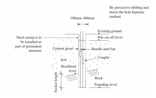
Micro-pile and mini-pile usually consists of one or a bundle of steel bar respectively encased by cement grout inside a borehole ranging from 100mm to 400mm in diameter. They are normally designed to be socketed into rock and are mainly used in small site area and for lighter structure. Steel casing are to be provided to support the borehole within the soil and/or fractured rock during drilling operation.
