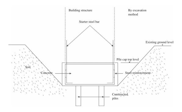
ELS works are carried out beforehand to facilitate pile caps construction works. Pile caps are built on top of a pile, or a group of piles to transmit the load. Pile caps are considered part of the foundation and substructure construction. Piles are first inserted into the soil followed by the pile caps construction. As a final step, concrete is poured to form a slab as the bottom of the basement.
