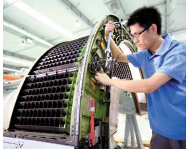
Maintenance on a D-Duct of a Boeing 777 T800 thrust reverser performed by HAECO Spirit AeroSystems.
