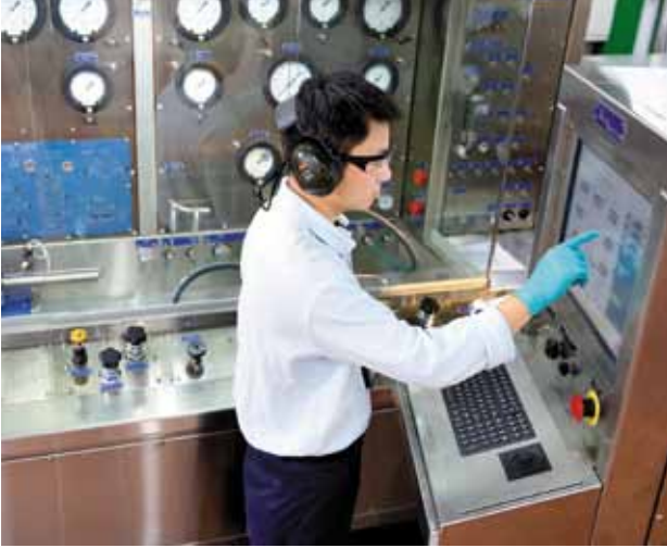
The new universal hydraulic test bench at the HAECO Component Overhaul (Xiamen) workshop.
