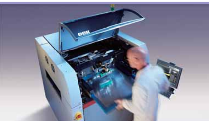
The DEK NeoHorizon is highly modular in design, enabling customers to configure two printers to form a highly flexible dual-track solution when needed
