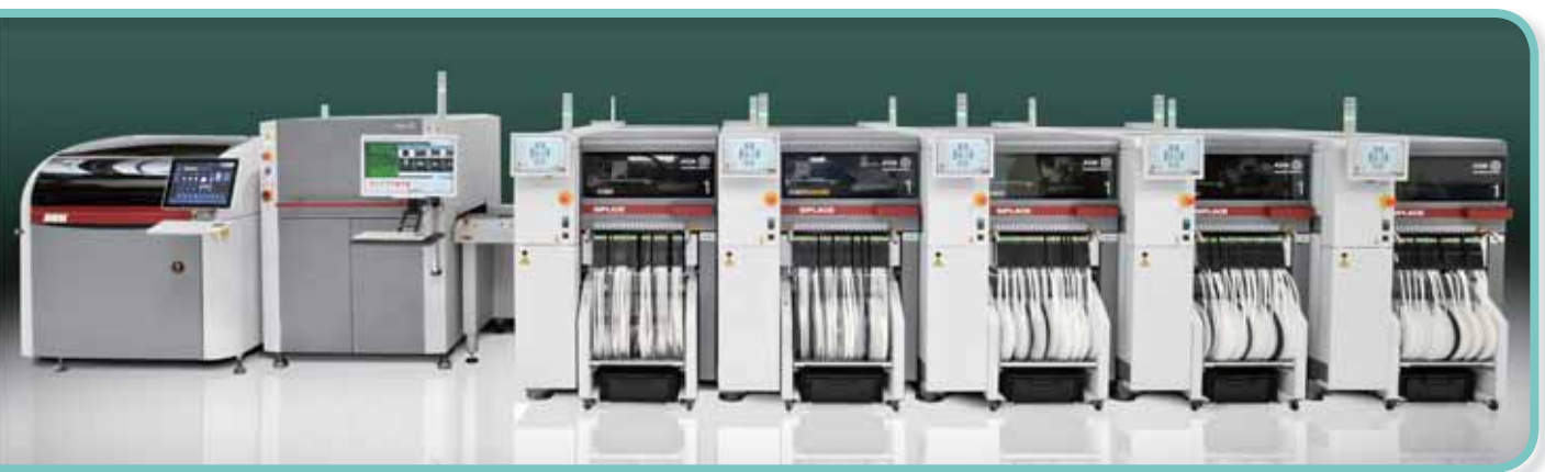
Introduced a closed-loop line solution comprising printing, solder paste inspection and placement solutions in the SMT production
