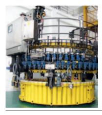
The dedicated device for opening/closing head cover of a reactor pressure vessel functions vitally by synchronized pulling of all the main bolts, i.e. unscrewing/screwing the main nuts to indirectly screw up/screw down the main bolts while guaranteeing the sealability of the pressure vessel. The whole process is timesaving, efficient and economical.
