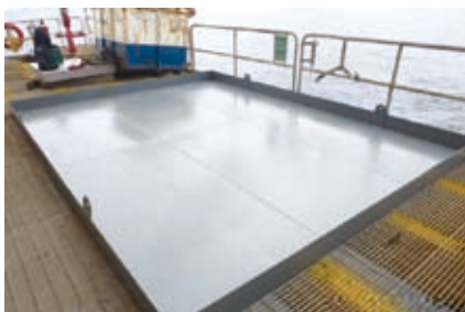
Specific temporary corner of debris collecting plates for preventing from oil spill
