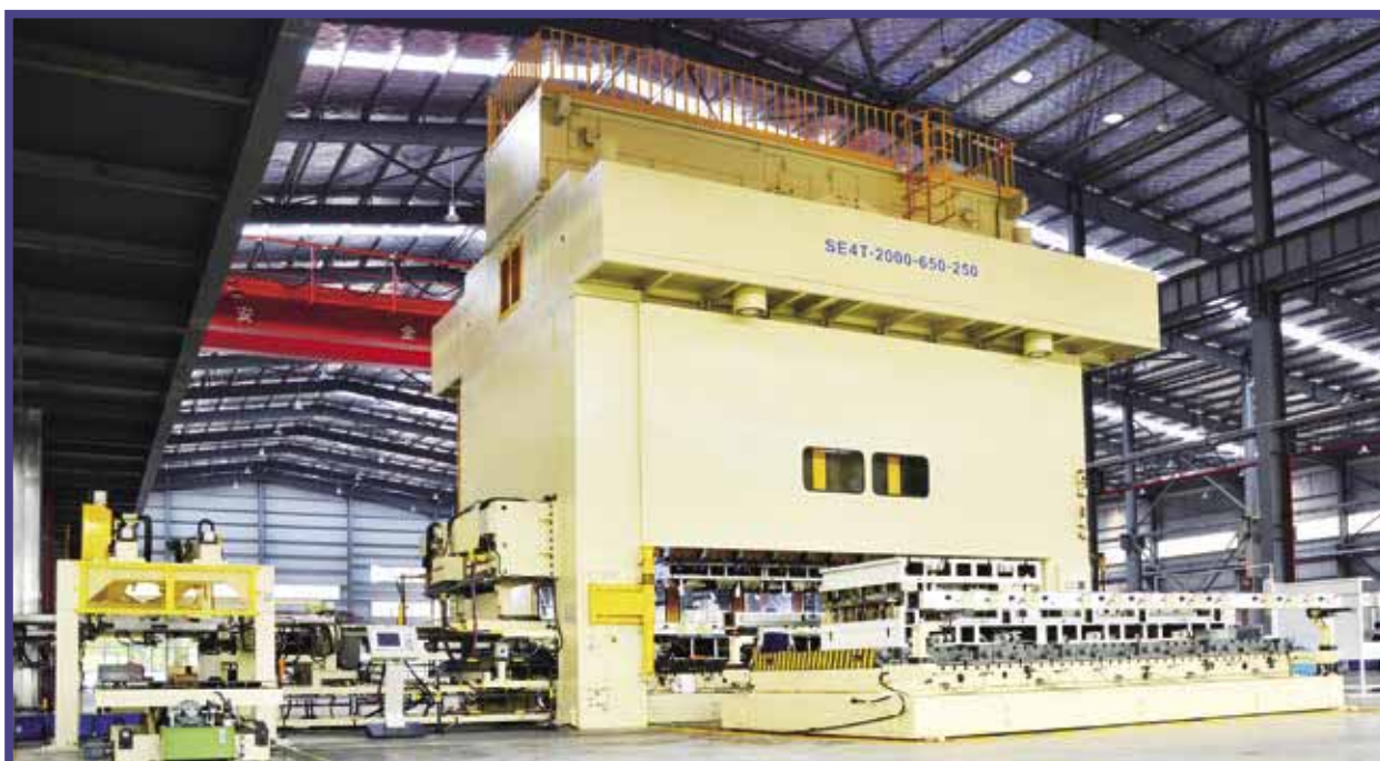
2,000 tonnes stamping machine for automobile components located at Digidie Guangdong (Zhongshan) Automobile Industrial Park
