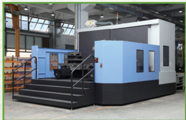
▲ Machine centre for machining high precision required casting products
