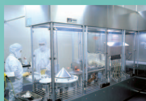
Beijing Tide's small volume injections production line
