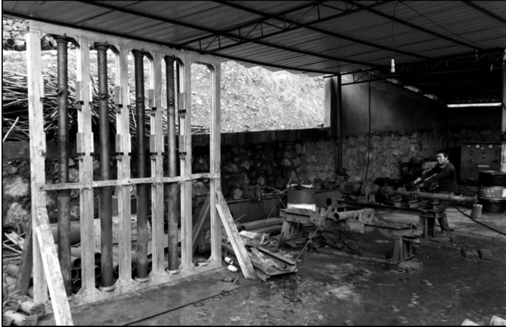
Figure 13-5: Maintenance Work and Testing of Hydraulic Supports in Lasu
