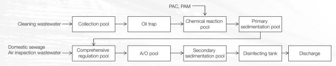
The processing capacity of the sewage treatment facilities in the plant area is over 100 tons/day. Wastewater after treatment reaches the quality standards issued by relevant departments without adverse effects to the surrounding water environment.
