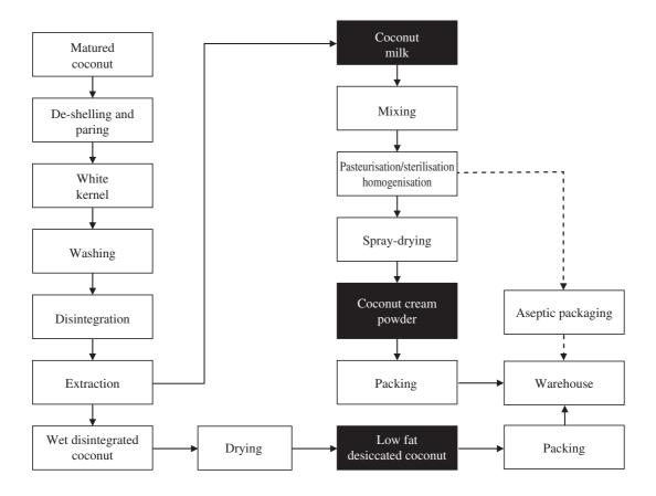
Note: The dotted line indicates the new processes involved in the production of coconut milk products.
