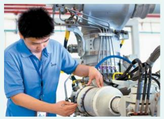
Based in Xiamen in Mainland China, HAECO Landing Gear Services completed its first repair and overhaul of Boeing 747-8 landing gear in 2017.
