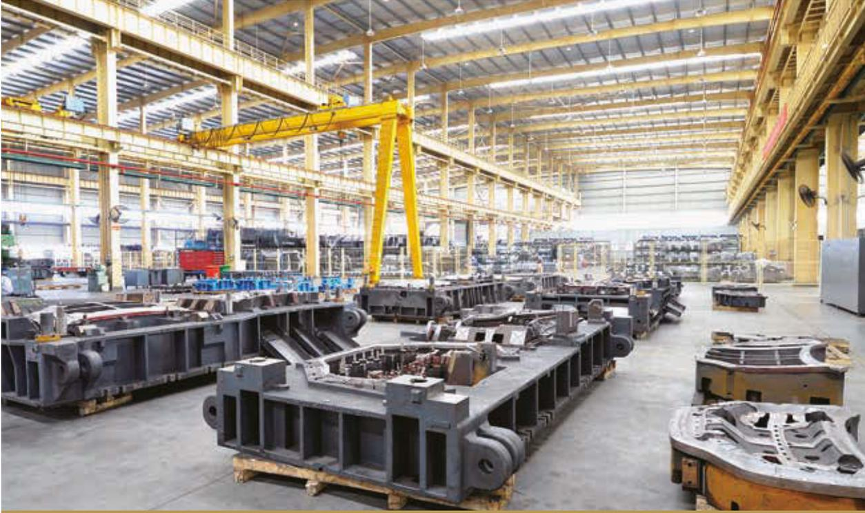
Workshop for automobile moulds used for high tensile autobodies
