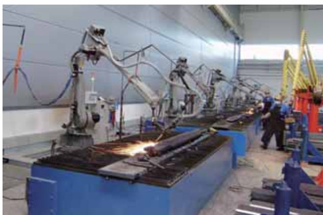
Photo: Imported robots mainly for cutting the bevel of big components such as cover plate and roof
