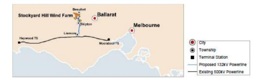
At the site there are both plains and hills, and the elevations are between 320m and 440m. The annual average wind speed at 110m above the ground is 7.8m/s as assessed, and the project's capacity factor will be about 42.1%, meaning good wind resources there. It is planned that the wind turbines for the project will be arranged at 149 places.
