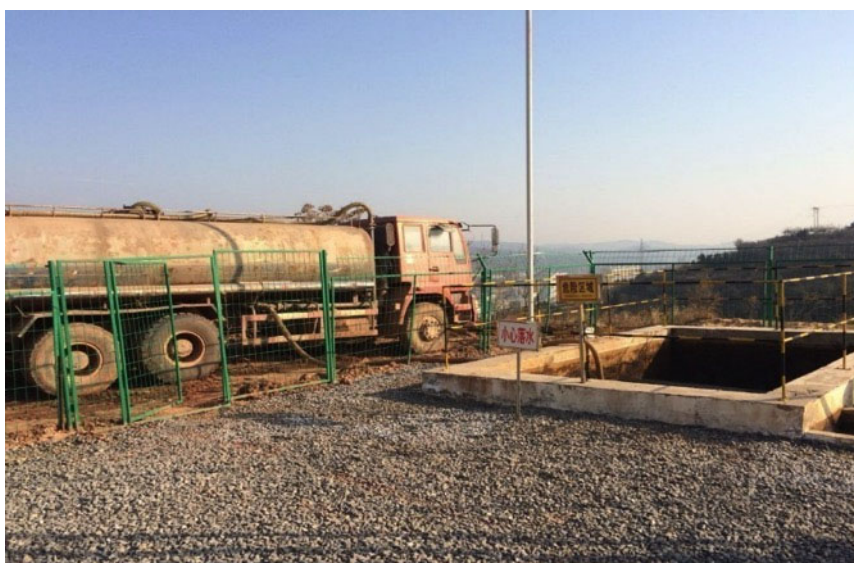
Transporting pumping water to fracturing well sites by water tanks 利用水罐車將排採水運輸到壓裂井場
