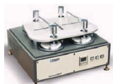
Martindale abrasion machine to evaluate abrasion resistance of textile materials
