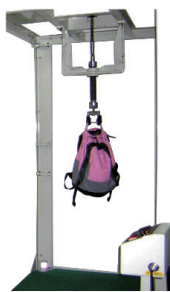
Bag handle jerk tester to test the strength of buckle and overall structure of finished goods
