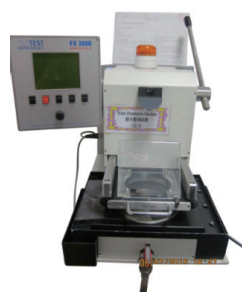
Waterproofness testing machine to test the waterproof level of raw materials
