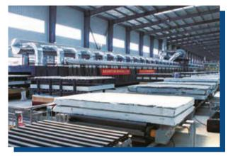
produced by the mine is used to produce a new type of building materials (i.e. foamed ceramics), which are mainly used as external wall insulation board and interior wall board due to its light, fireproof, anti-flaming, moisture-proof, insulation, sound-proof and other properties, and can be used as a new wall materials to replace the existing wall materials in the domestic market and has huge market potential.
