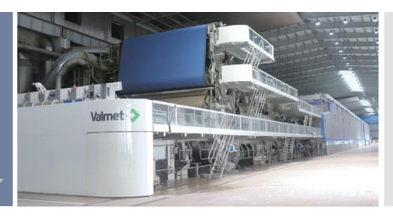
During the Year, PM2(VN) at the Vietnam base commenced production in August 2017 and went into commercial production in January 2018. With an annual design production capacity of 350,000 tonnes for linerboard products, this new paper machine has brought the Group's total annual design production capacity to 14.08 million tonnes.
