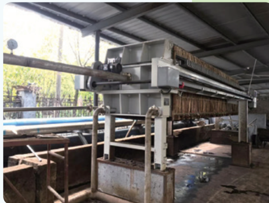
Yongsheng Dyeing's high pressure diaphragm filter press 永盛染整的高壓隔膜壓濾機
