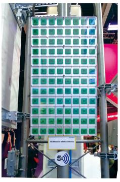
5G Massive MIMO antennas have been successfully deployed for trials globally
