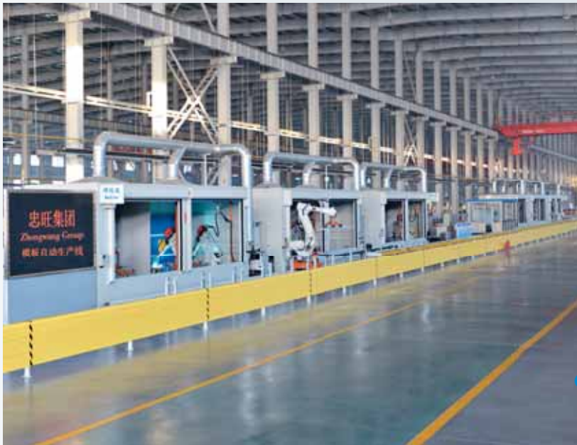
Automatic welding production line for aluminium alloy formwork
