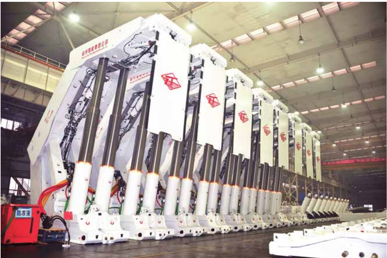
8.8m Hydraulic Roof Support, independently developed and manufactured by ZMJ 鄭煤機自主研製製造的8.8m液壓支架
