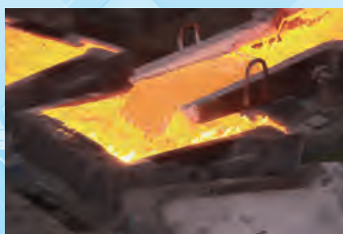
CCS successfully poured the first anode plate
