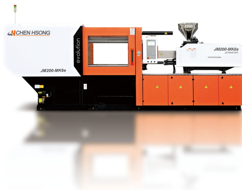
捷霸MK6e伺服驅動注塑機 JETMASTER MK6e Servo Drive Injection Moulding Machine
