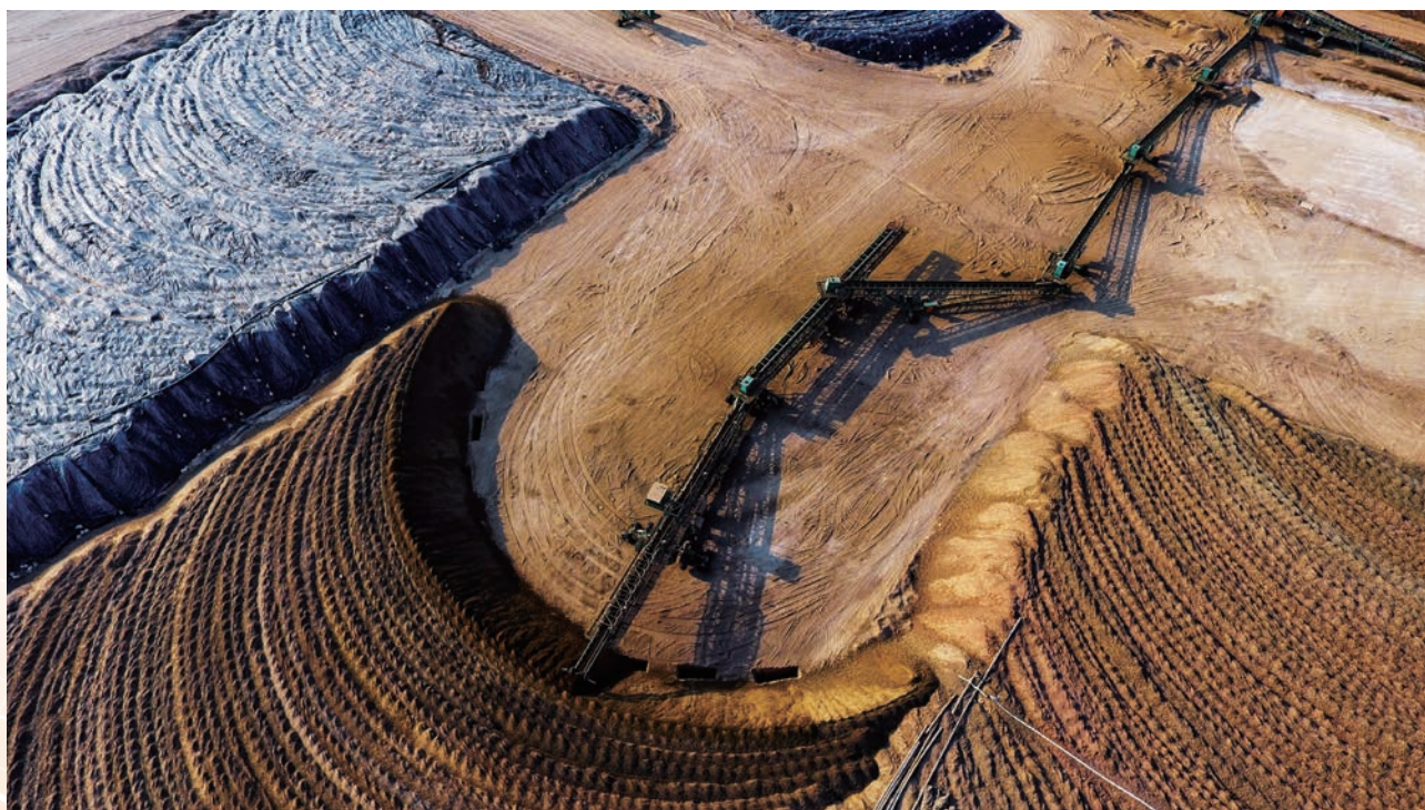
A bird view of heap leaching at Luanshya
