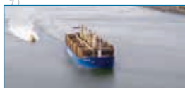
Imabari Logger is a versatile ship designed to carry logs and a wide range of bulk and breakbulk cargoes
