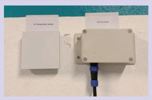
IoT System and CO & Temperature Sensors
