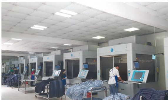
Texhong Thai Binh Garment: laser technology equipment 天虹太平服裝：激光技術設備
