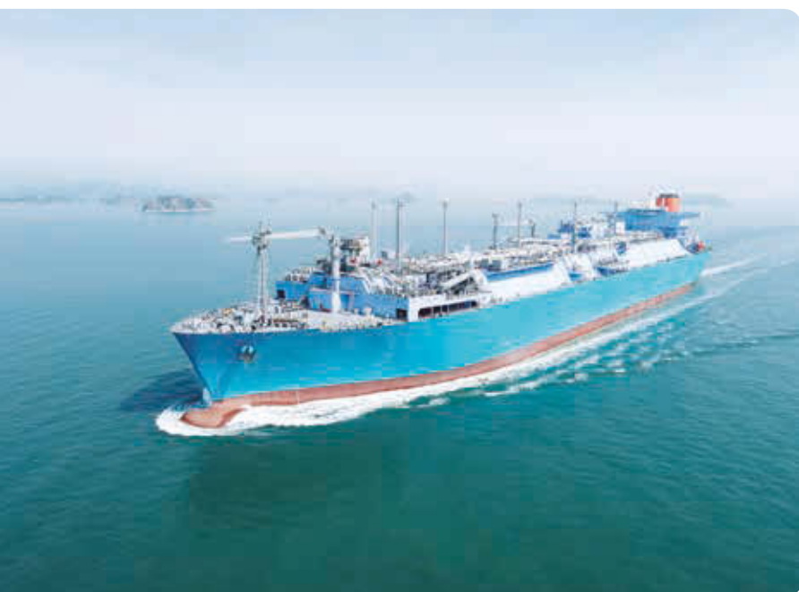
▲ The FSRU vessel equipped with LNG tanks and regasification equipment in the offshore LNG terminal project.
