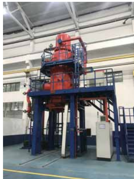
A vacuum quenching furnace in a heat treatment workshop at one of our factories in Ningbo.
