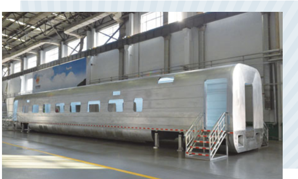
Aluminium alloy body for "Fuxing EMU" high-speed trains
