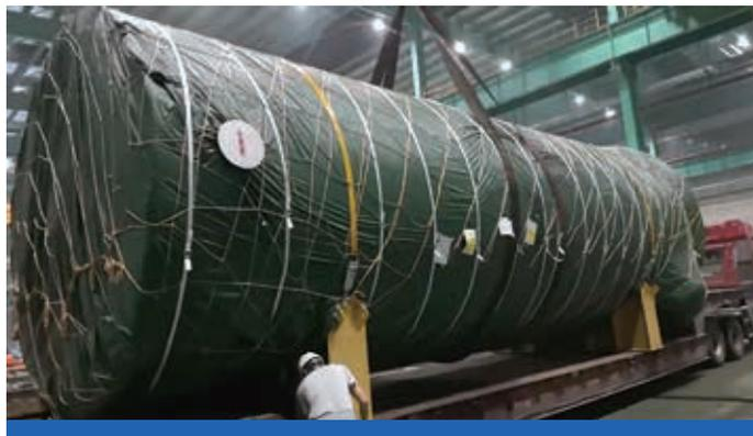
The project was designed by Air Liquide, while Jingjiang Daming Heavy Industry has provided the “one-stop” processing services of high standard cutting, grooving, rolling, welding and seamless inspection. All processes were finished strictly in accordance with customer standards and were finally examined and accepted.
