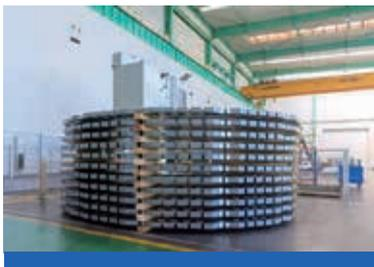
3. *Jingjiang Daming Heavy Industry supported pumped-storage power station with magnetic yoke steel processing*
