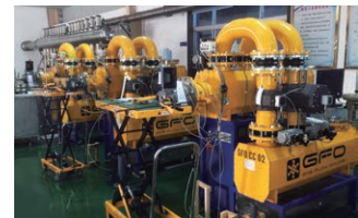
Gas flow standard device by standard meter method
