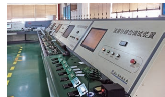
Integrated commissioning device for flowmeter
