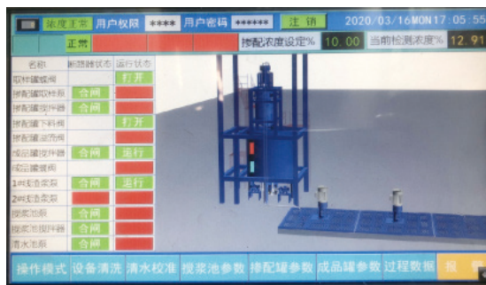
Real-time monitoring screen of seriflux recycling system 漿水回收系統實時監控畫面
