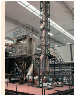
Discharged air generated by rotary kilns in magnet production is acidic
