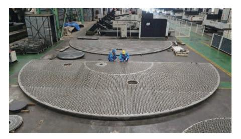
A tube sheet with the longest diameter in the world at present that was manufactured and processed by the Machine Processing Division of Daming Heavy Industry for a paper project of Valmet has been successfully shipped to Brazil.
