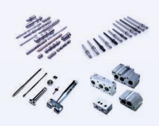
Precision machining is the second largest business segment of the Group which accounted for 31.7% of the Group's revenue for the year ended 31 December 2020. It is a process that involves using computer numerical controls and other machines and tools to drill or shape metal components with highly precise specifications used in various finished products. Precision machining is performed on bar stocks and other formed materials sourced from global thirdparty suppliers.
