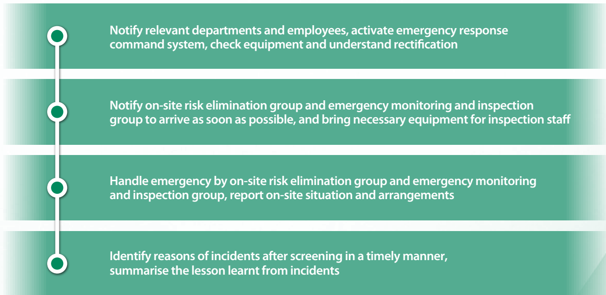
General Procedures for Emergency Response
