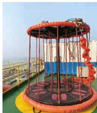
The offshore production units of the Drilling Division are fully equipped with rigid cages. In the process of personnel transfer, the rigid cage support rods can effectively avoid the cage and personnel swinging caused by the hull due to swells, and improve the safety of hoisting operations for staff ascending to and descending from the drilling rig on shift change for application ships.
