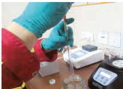
Each operation unit under the Drilling Division is equipped with a portable domestic sewage COD detector, and the domestic sewage is regularly sampled and tested to ensure that the discharge meets the standard
