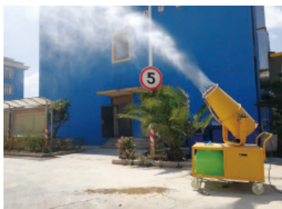
Picture of an operating fog cannon 霧炮機工作畫面
