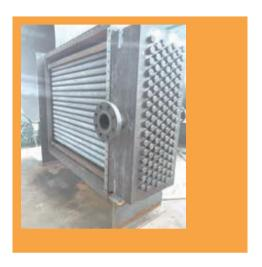
8. Daming Heavy Industry manufactured stacked heat exchangers to serve a 600,000-tonne ABS and AS project
