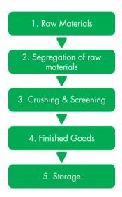
Chart: Construction waste recycling flowchart
