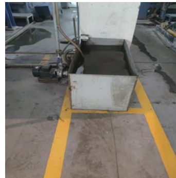
Recycle the cooling water discharged from the equipment 回收設備排放的冷卻水
