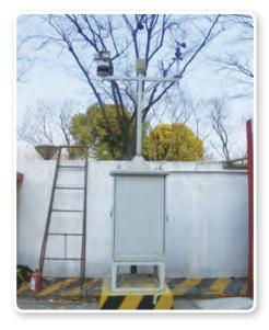
Noise dosimeters are installed at construction site to monitor noise level. Meter reading is recorded few times a day at random intervals serving as random inspections.
