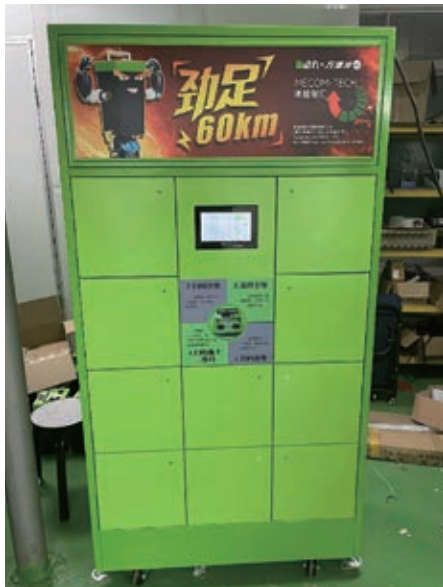
Charging cabinets for battery-swapping systems
