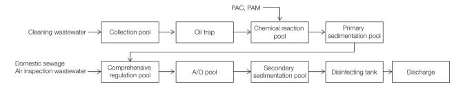
The processing capacity of the sewage treatment facilities in the plant area is over 100 tons/day. Wastewater after treatment reaches the quality standards issued by relevant departments without adverse effects to the surrounding water environment.
